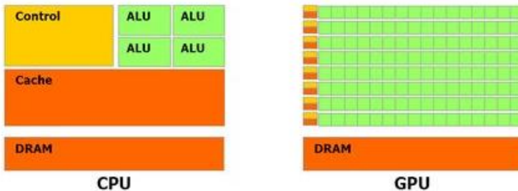
Figure 3.2: GPU vs CPU memory hierarchy [15]
