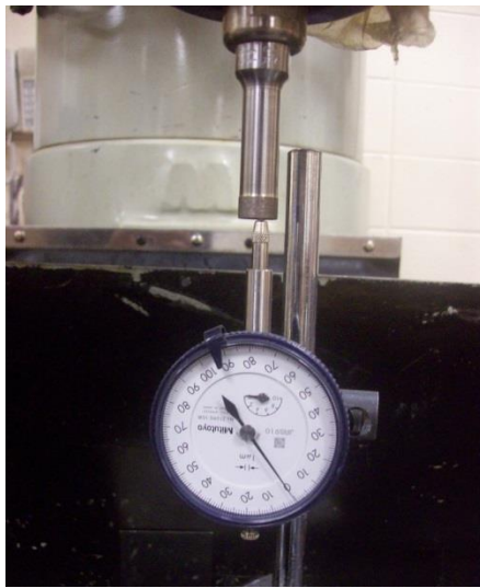
Figure 118: Dial gage placed under the drill bit and in contact with the surface as it operates and measure the wave amplitude
