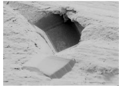
Figure 1: Diamond pull out due to weak mechanical locking inside the matrix
