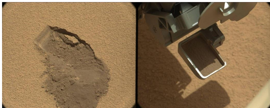
Figure 13: Mechanisms for scooping, sieving and portioning samples of powdered rock and soil samples, JPL
