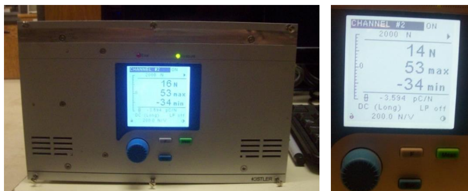
Figure 115: A/D converter received signal from dynamometer of the applied force
