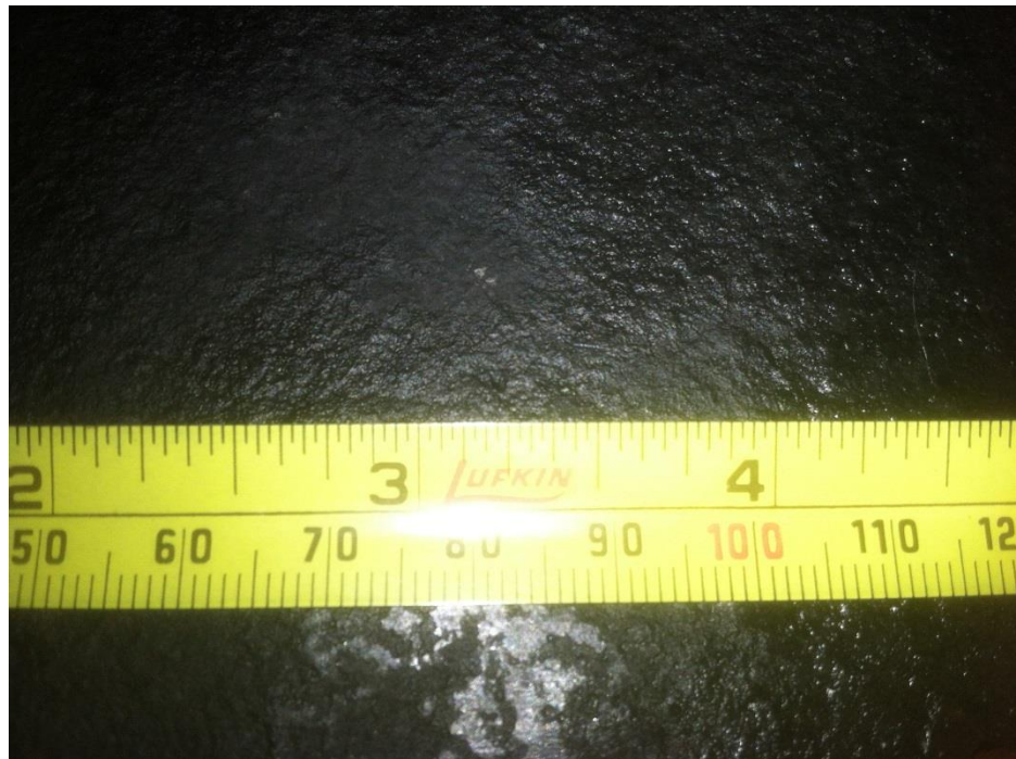
Figure 79: Side view of basalt sample close up image showing an estimated grain size and porosity level
