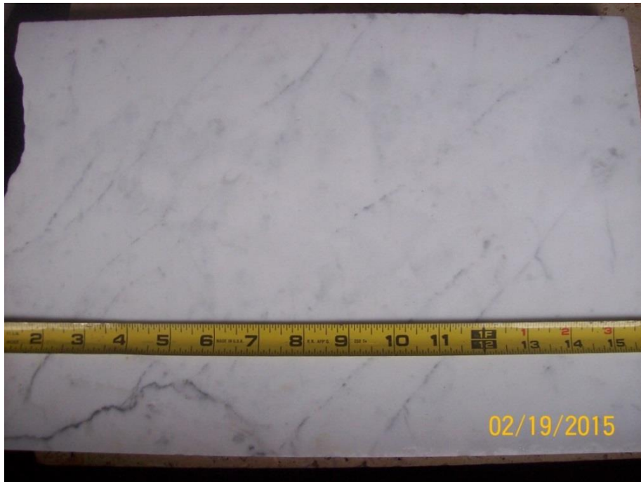
Figure 76: Top view of marble Rock Sample with overall dimensions of 25x152x2.54 cm
