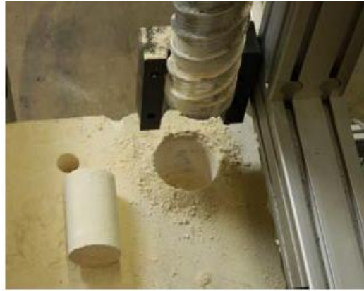
Figure 46: Using the Auto-Gopher, the first core (57.25 mm diam. and 97.25 mm long) that was produced of limestone (photo courtesy of K. Zacny, Honeybee Robotics).
