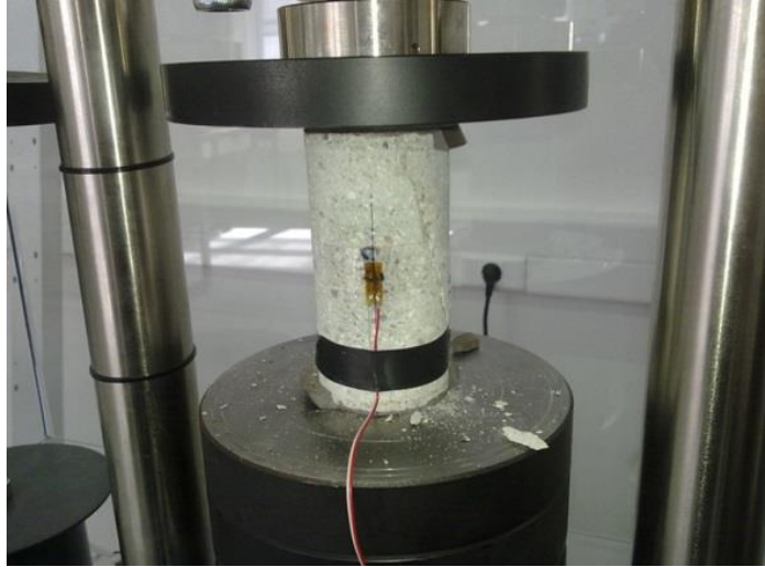
Figure 86: Typical Uniaxial Compression Strength test setup (UCS), National Technical University of Athens
