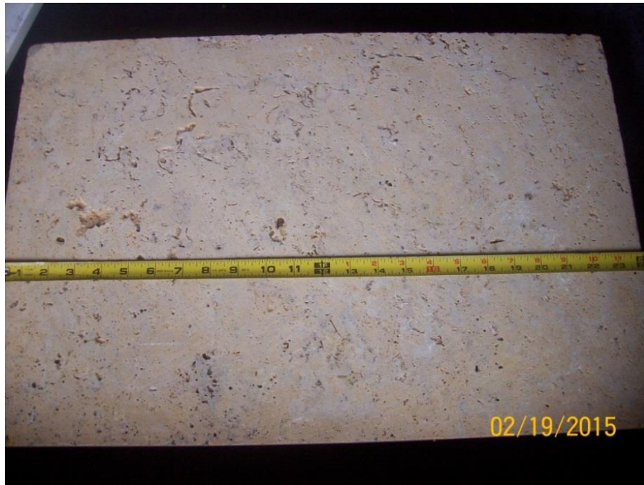
Figure 74: Top view of travertine Rock Sample with overall dimensions of 38x60x2.5 cm
