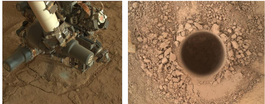
Figure 12: Mars Hand Lens Imager (MAHLI) camera on NASA's Curiosity Mars rover shows the first sample-collection hole drilled in Mount Sharp, JPL
