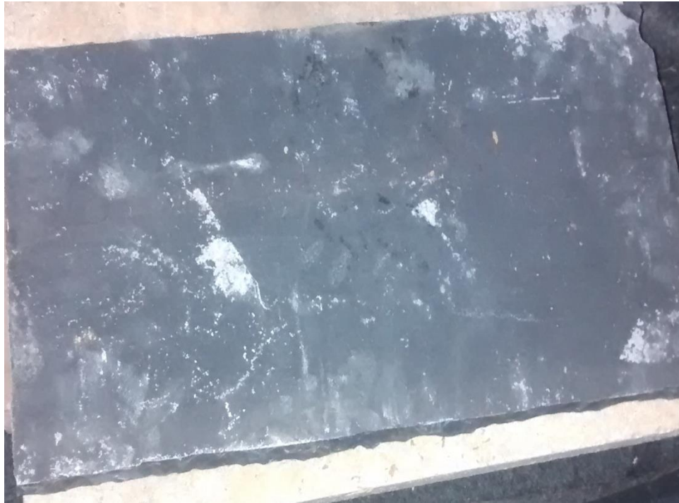
Figure 78: Top view of basalt rock sample with overall dimensions of 30x58x3.8 cm
