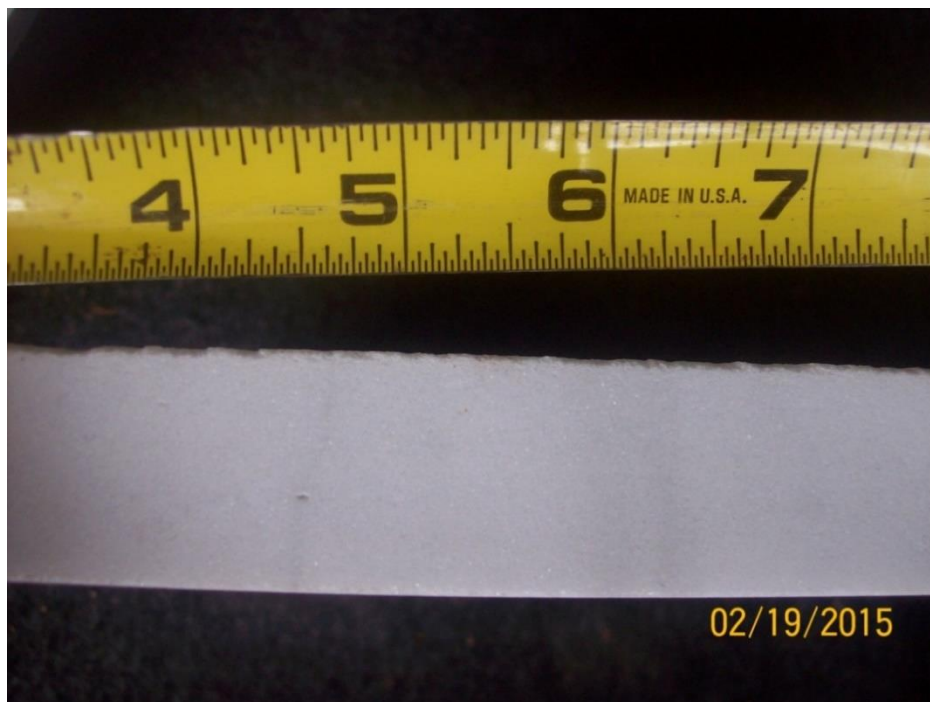
Figure 77: Side view of marble sample close up image showing an estimated grain size and porosity level
