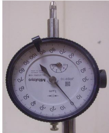
Figure 117: a) Amplitude measuring device, dial gage, b) Typical drill bit showing tuning length (Weilong Cong, 2013)
