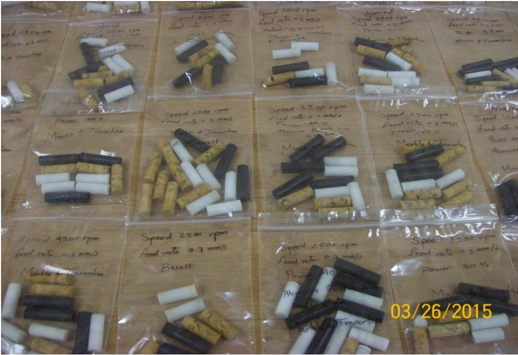
Figure 125: Rock samples drilled at various input parameters close up view showing the labeling system applied to identify each core sample.
