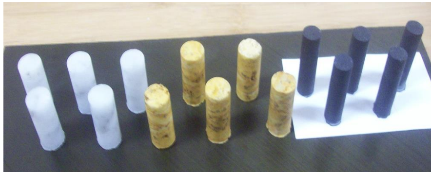
Figure 104: Specimens prepared for Vickers hardness tests
