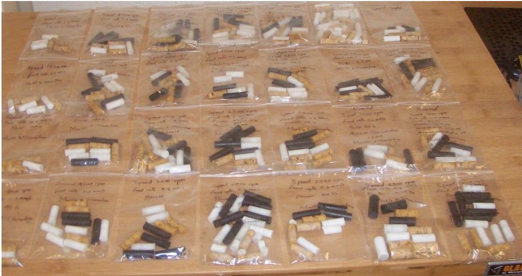
Figure 124: Experimental core rock samples drilled at various drilling parameters
