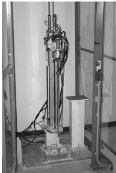
Figure 22: Test equipment with integrated drill/core tool that is 70 cm long. ESA and Galileo Avionica
