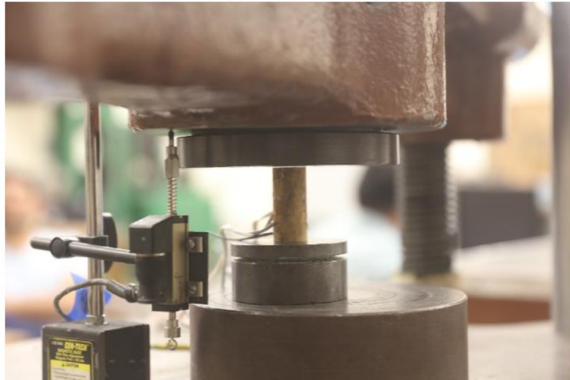
Figure 97: Rock specimen in UTM (spherical swivel at the bottom)
