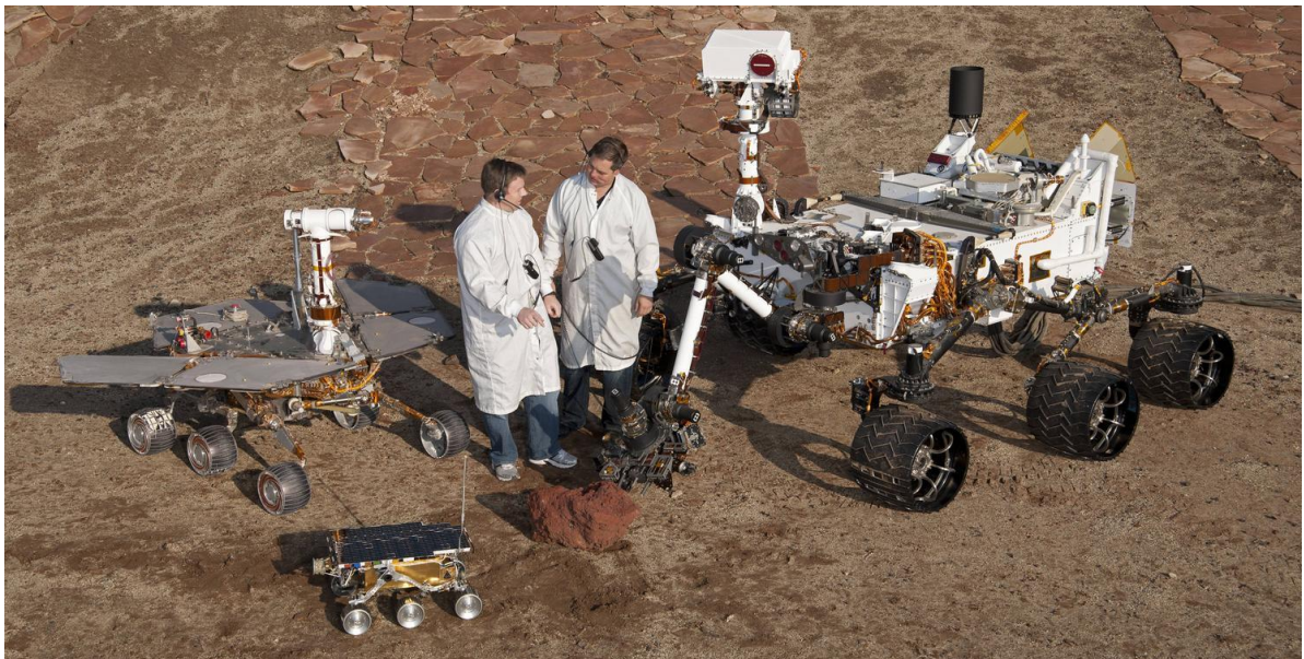
Figure 4: Size comparison between three generations Mars rovers landed on Mars between 1997 and 2012, Mars Exploration Rovers, JPL
