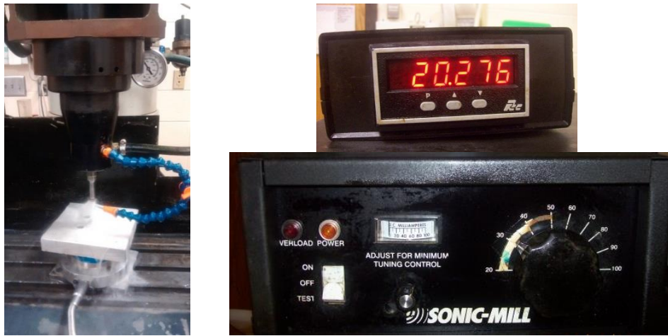
Figure 114: Dynamometer measuring applied force (left), ultrasonic frequency display unit by Sonic-Mill (right)
