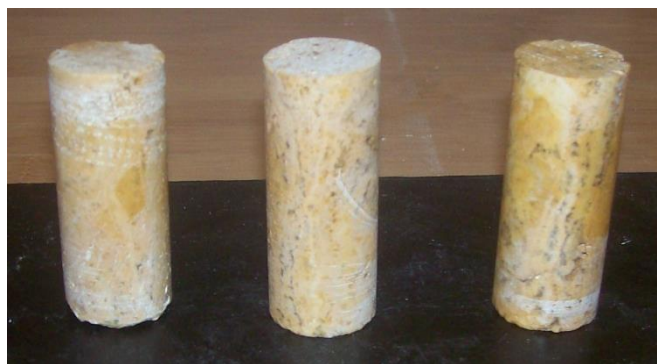
Figure 87: Travertine specimens (3) prepared for compression test
