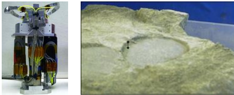
Figure 8: Rock Abrasion Tool (RAT) on Spirit & Opportunity Rovers (left) and an exposed fresh rock surface (right), Mars Exploration Rovers, JPL
