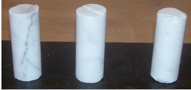
Figure 88: Marble specimens (3) prepared for compression tests
