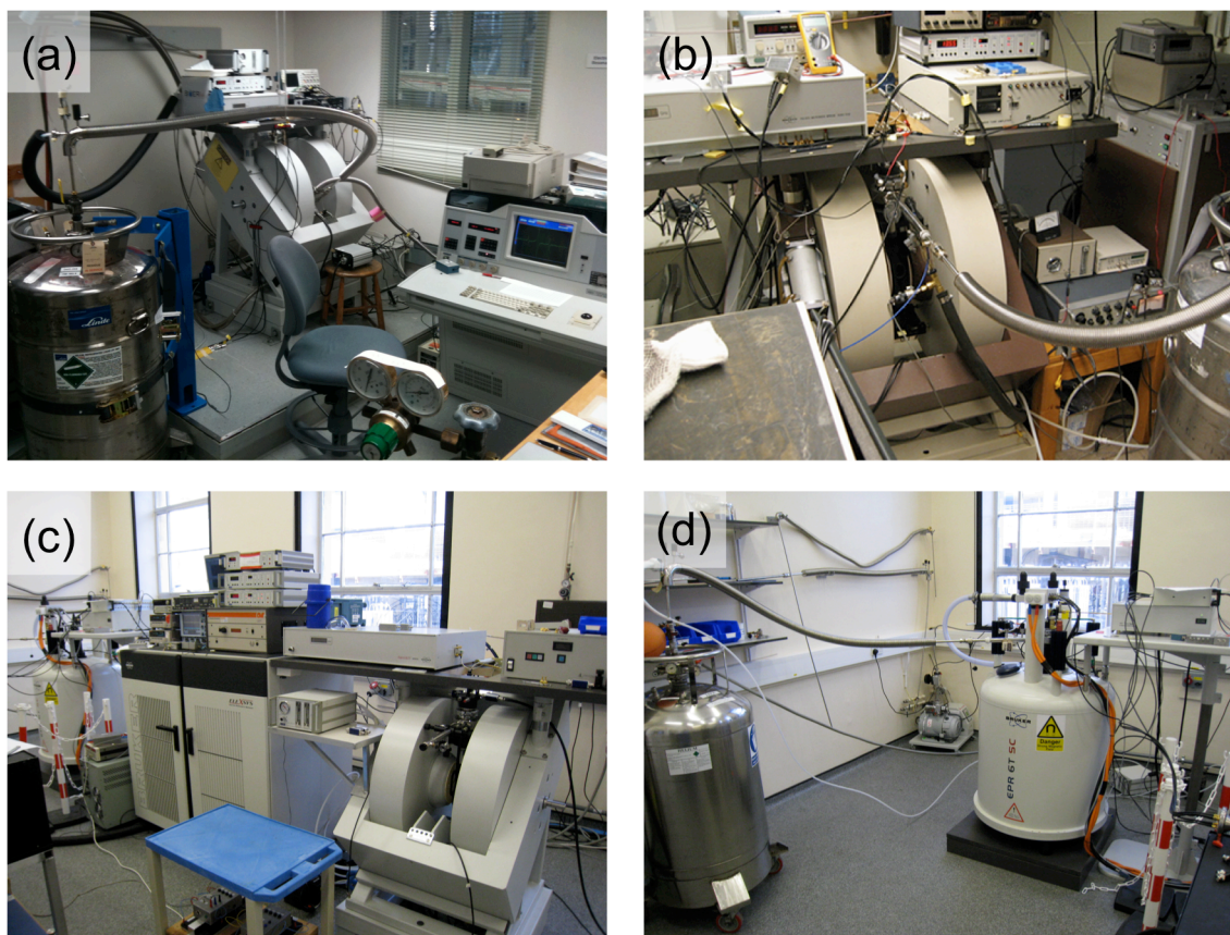
Figure 3.3: EPR spectrometers used in this work: (a) Bruker ESP300E X-band cw-EPR set-up at BIERLab, LBNL. (b) Bruker ElexSys E5801 X-band EPR spectrometer at Princeton. Bruker ElexSys E680 with (c) X-band electromagnet (right unit), and (d) W-band superconducting magnet at Oxford.
