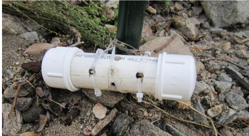
Figure 2: HOBO house deployed (Bull Control)
