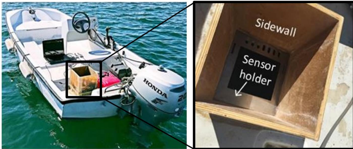
Figure 4. Modified boat with a well and sensor system holding plate to conduct.
