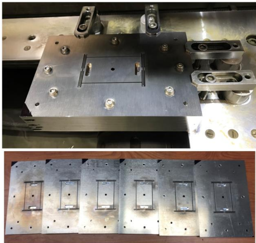
Figure 10. Post-cutting stage of six-plate cutting test mounted on wire-EDM (top). And the resulting individual plates splayed out (bottom).
