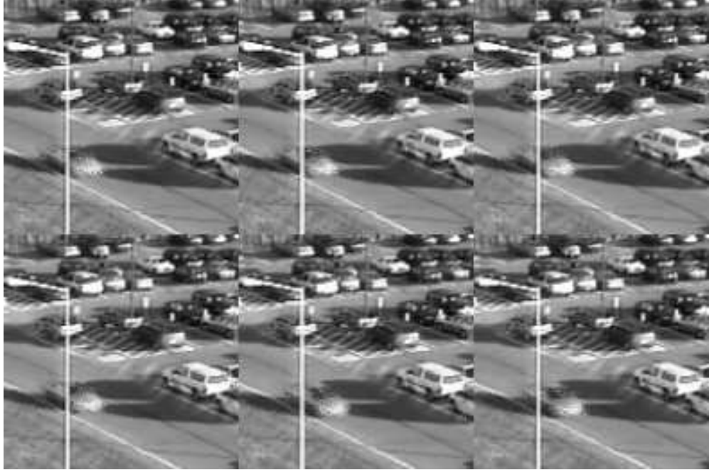
Figure 2.7: The reconstruction results of six consecutive frames compressed by our algorithm. The PSNRs for the first row starting from the left is: 33.7896 35.7451 36.1793 and the PSNRs for the second row starting from the left is: 33.7118 32.6931 34.7961.
