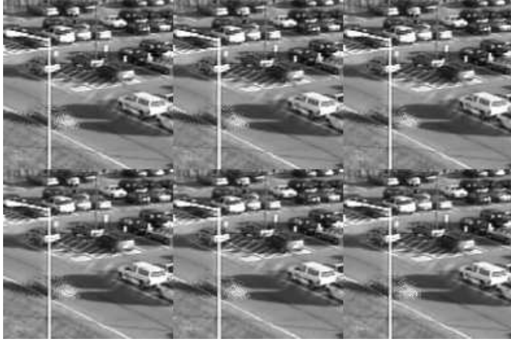
Figure 2.8: The reconstruction results of six consecutive frames compressed using a fixed rate, chosen to match the average compression rate of our algorithm. The PSNRs for the first row starting from the left is: 32.5228 33.9217 34.5397 and the PSNRs for the second row starting from the left is: 33.9049 32.0122 29.9636.
