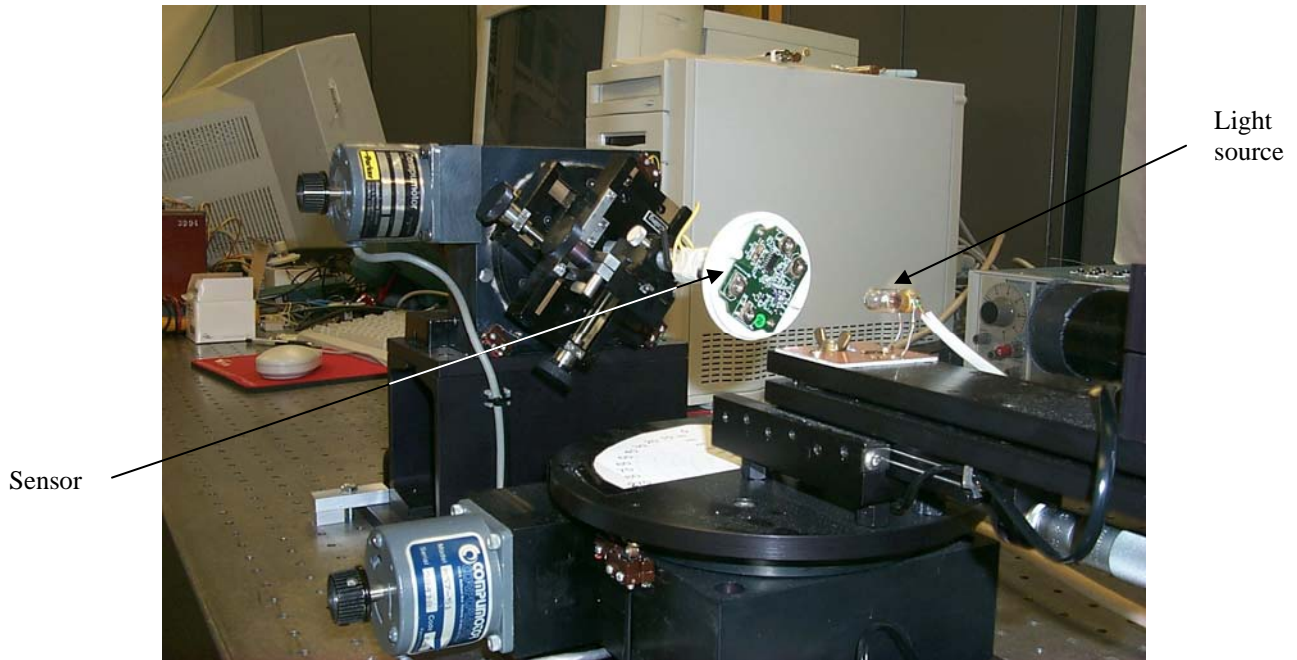
Figure 11- Sensor and light source position in spatial measurements (shown with the front cover of the sensor removed.)
