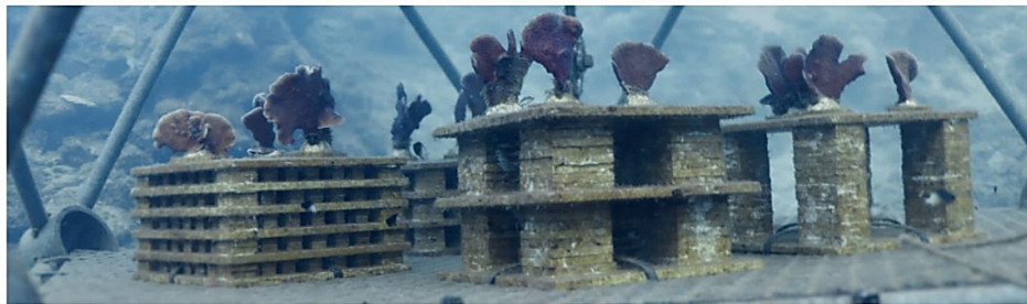
Figure S2.8 Limestone ARMS can be built with differing internal complexities. Smaller, more numerous internal components yield higher internal surface area, with implications on fouling (biofilms and sessile invertebrate communities) and a correspondingly lower internal surface area to volume ratio. ARMS complexities can be designed based on desired recruitment patterns, with higher complexity ARMS recruiting smaller mobile organisms.
