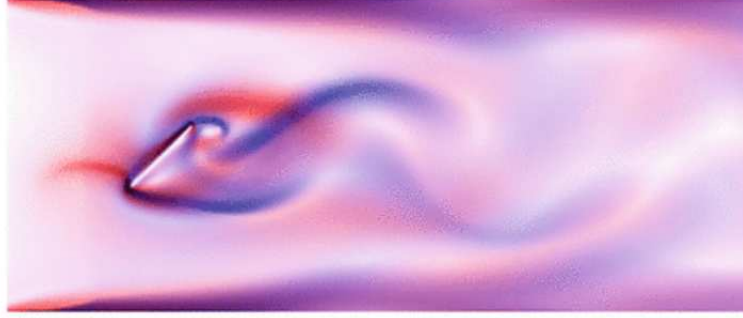
Figure 2.2: FTLE computed for a tilted bar data set with total integration time of 1.0 second. From Schneider et al. [79].
