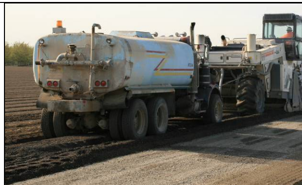
(a) Rotary mixer/recycler coupled to water tanker
