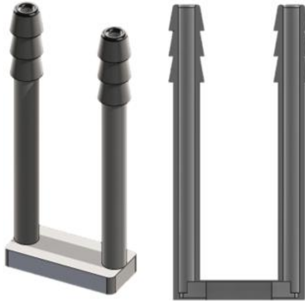
Figure 3.1 CAD model of SCI-OTD with tube fittings designed to extend past the skin and outside the animal
