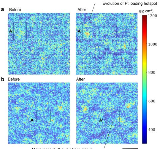
Movement of Pt away from cracks
