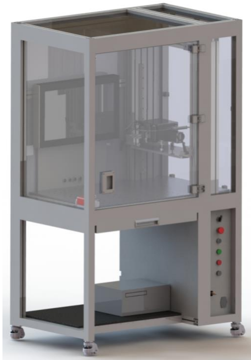
Figure 4 – Solid model of the bespoke milling machine used for the slotting measurements
