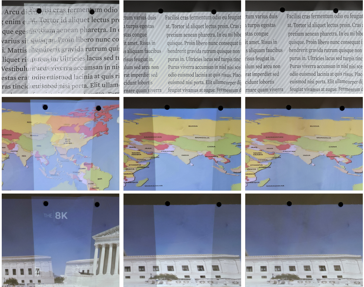
Figure 5.8: Results of our calibration, rendering and display method. Left column : No calibration. Middle column : Calibrated result without blending. Note the accuracy of our registration. Right column : Our final blended result.
