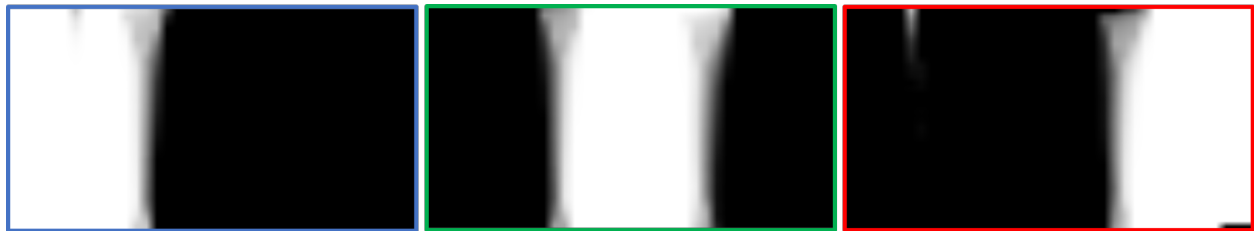
Figure 5.6: The projector blend masks in (u, v) space. Note that each mask represents the entire display region.
