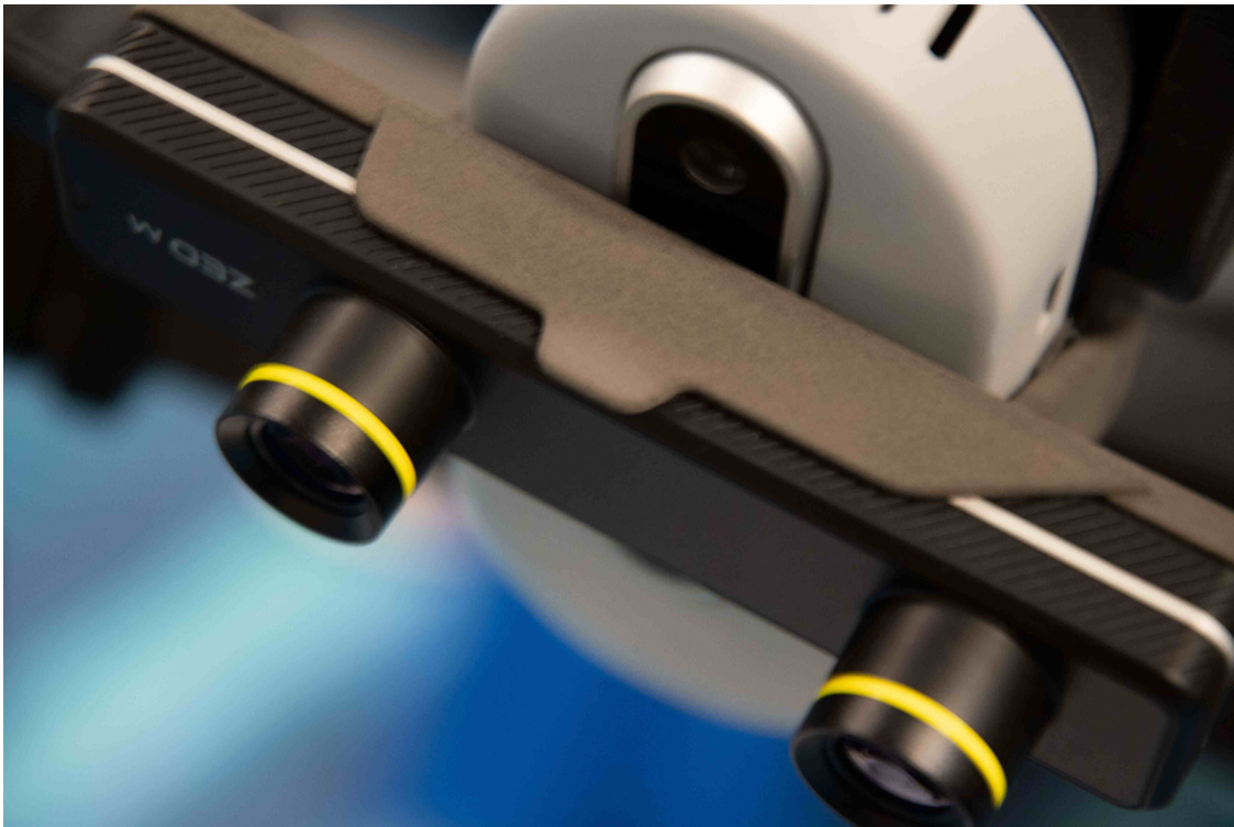
Figure 4.6: ZED Mini mounted on the Stretch RE1’s head. The ZED Mini was used to simulate the operator’s gaze and to provide stereoscopic vision to the operator.
