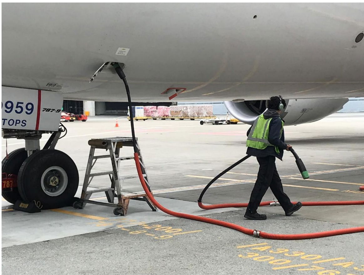
Figure 32: Ground crew worker disconnects a GP cable from a 787-900 which requires 2 GP cables for higher current supply (Achatz Antonelli, 2019)
