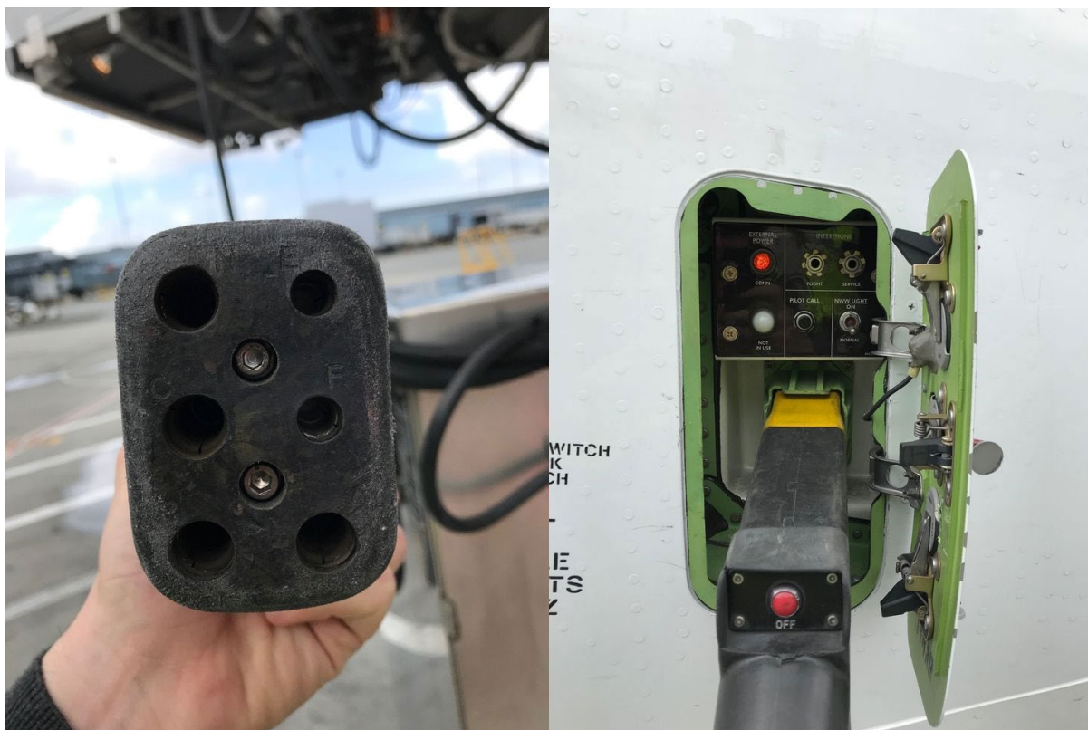
Figure 31: GP connector and receptacle at SFO international airport (Achatz Antonelli, 2019)
