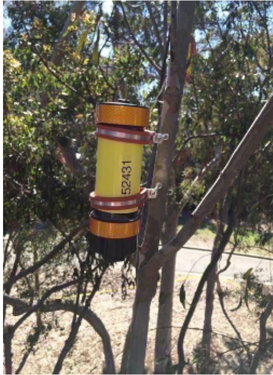
Figure 3.6. Tree mounted G-LINK_LXRS-2G-M 3-axis accelerometer
