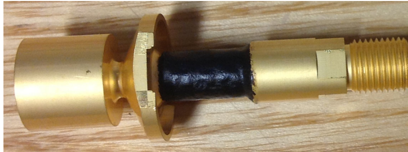
Figure 9.19: Rubber is added around the cavity flexture to increase damping and minimize ringing.
