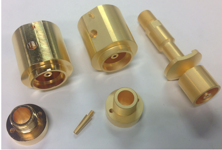
Figure 9.4: Some gold-plated aluminum pieces from two different batches. The shiny pieces on the left are from a run that left \sim 20\% nickel in the gold. The dull pieces on the right are a 24 carat plating, specified to be 99.9% gold.
