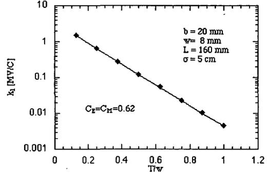
Figure 4: Loss factor for a rectangular slot vs.  $T/w$  ratio. The black diamonds are MAFIA points.
