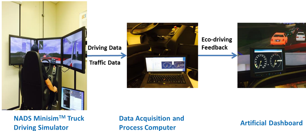
Figure 8. Integration of truck EAD system with truck driving simulator
