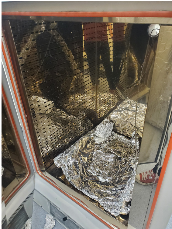
Figure 3.3: Inside of Despatch oven used to bake the vacuum chamber
