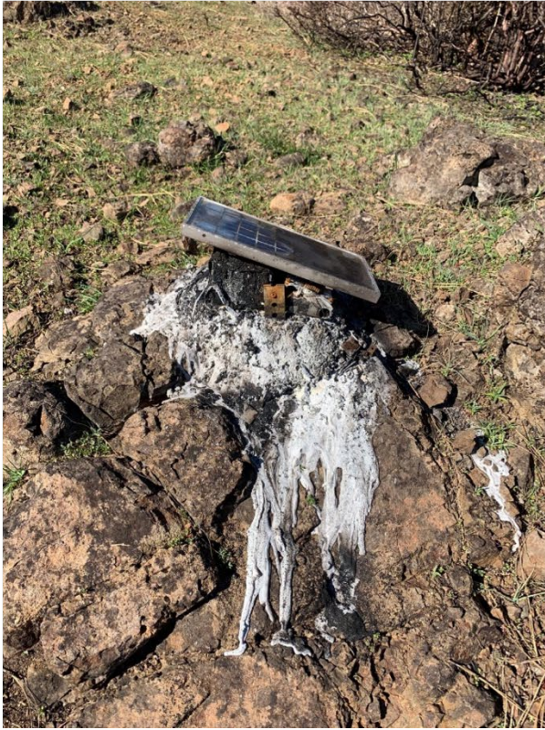
Temporary stations that sustained damage in the field: (a) station destroyed during a recent fire, and (b) station run over by a truck.
