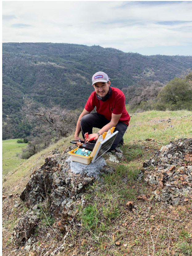
Site visit to a temporary seismic station at The Geysers geothermal field. During each visit SD memory cards were exchanged and the technical status of the stations was assessed.
