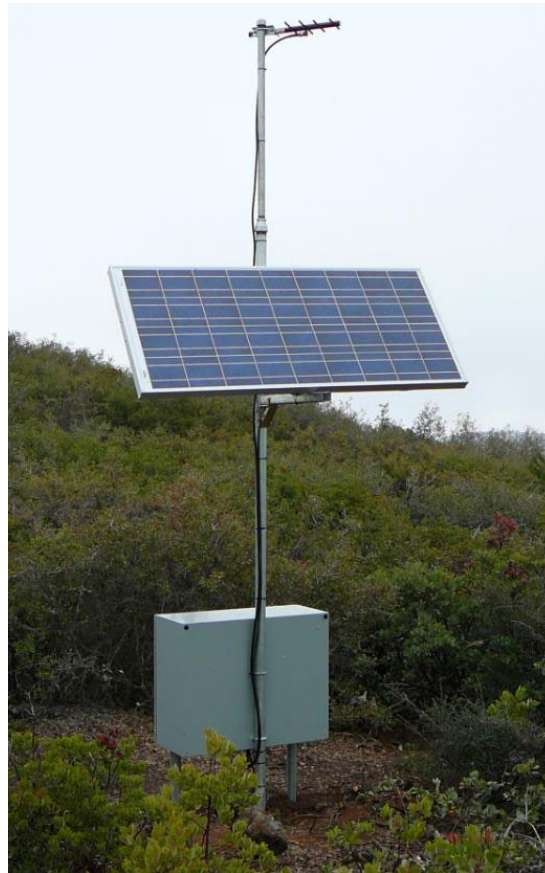
Site of a permanent seismic station at The Geysers geothermal field with antenna, solar panel, and box housing electronic components. The seismic sensor is buried at the foot of the pole.
