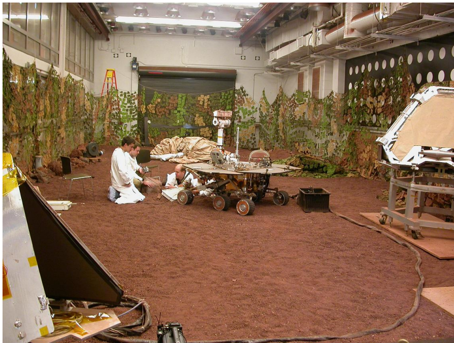
Figure 31 Rover in the sandbox with three mission members. To the right is the lander from which the rover emerged, once it arrived to Mars. In the upper left are the windows from which people can observe the position of the rover in the sandbox. During the PORT, signs were posted warning the MER mission scientists to stay out.
