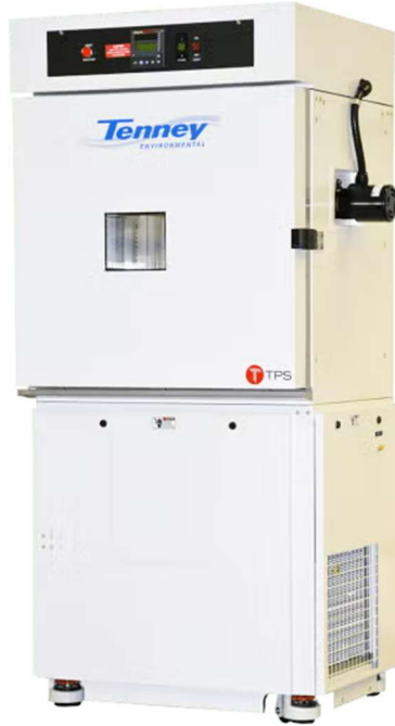
Figure 4. Tenney UTC Upright Temperature Chamber.
