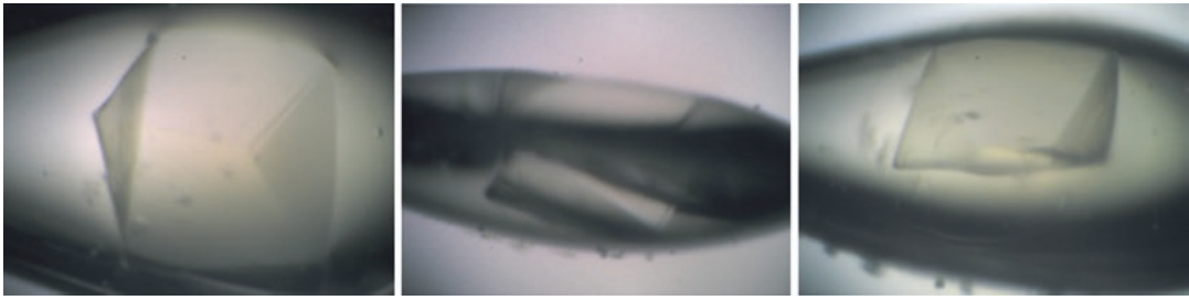
Fig. 1 Bright-field images at a synchrotron beamline of a mechanically well-centered T4 lysozyme crystal embedded in cryosolvent, viewed with 10 \times magnification. ( Left ) Goniometer \omega = 0^\circ – crystal seems well-centered; ( middle ) Goniometer \omega = 90^\circ – crystal seems split; ( right ) Goniometer \omega = 135^\circ – crystal seems too high. (Sample courtesy of B. Goblirsch, M. Wiener, University of Virginia)
