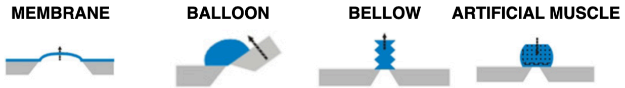
Figure 2.3: Types of elastic fluidic actuators. Image reproduced from De Volder et al [1].
