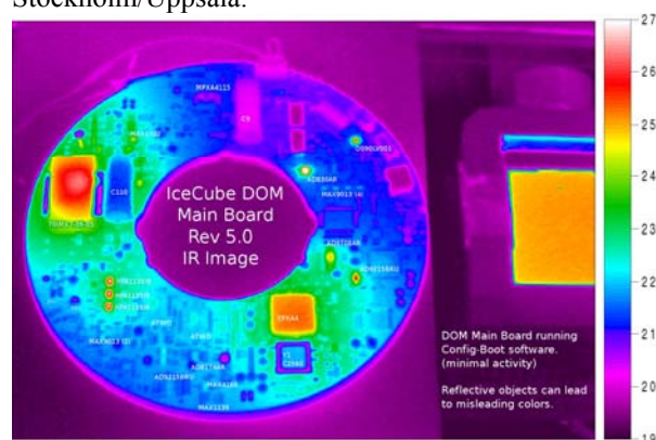
Figure 14. This is an infrared image of a DOM MB that was operating for about 40 minutes. The orange block on the right hand side is a reference temperature source in units of centigrade. Some of the objects in the picture appear colder because they reflect surrounding areas.
