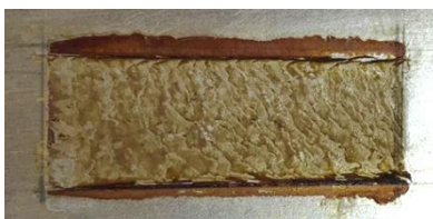
Figure 2.11: An example of a post-test coupon after heptane has been applied to remove the excess oil.
