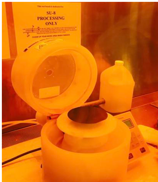
Figure 10. Wafer Placement on the Vacuum Chuck Spinner
