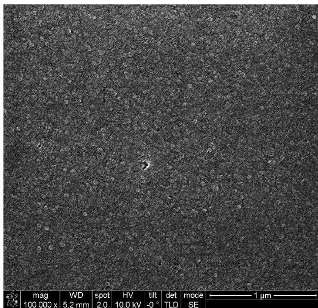
Fig 4.6- SEM image of ZnSnN 2 thin films deposited at the substrate temperature of 400 °C and vacuum annealed for 4 hours with N 2 /(N 2 +Ar) ratio of 50%. (SEM conditions are HV=10kV, WD=5.3 mm, spot size=3.0, and scale bar=500nm and 200nm).
