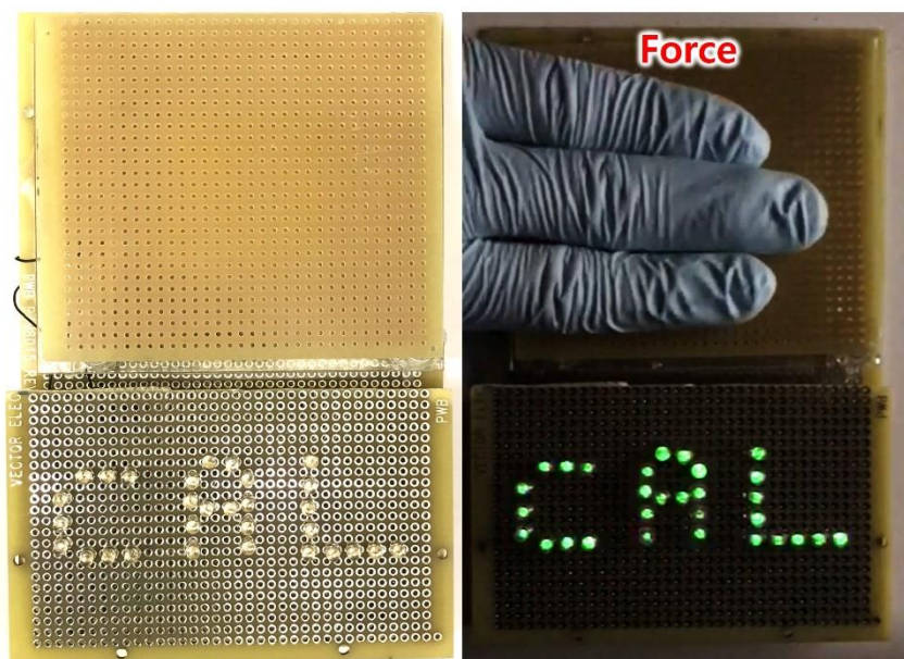
Figure 2-23. Photographs of 30 LEDs connected to the Tribo-PhD. The images show the LEDs when the room light was switched on (left) and off (right). Reprinted with permission. 2 Copyright 2021, American Chemical Society.
