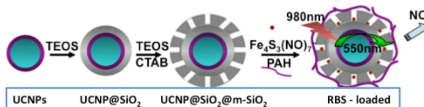
Fig. 19. Preparation UCNPs with a mesoporous silica shell impregnated with Roussin's Black Salt (red dots), a photo active nitric oxide generator, and coated with poly(allylamine). NIR irradiation leads to upconversion to wavelengths overlapping the RBS absorbance and NO uncaging [53]. ( Needs Permission ) Question: has this been obtained?
