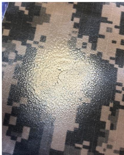
Figure 4S.26. Optical image of UiO-66-NCS spray coated on Nyco fibers.
