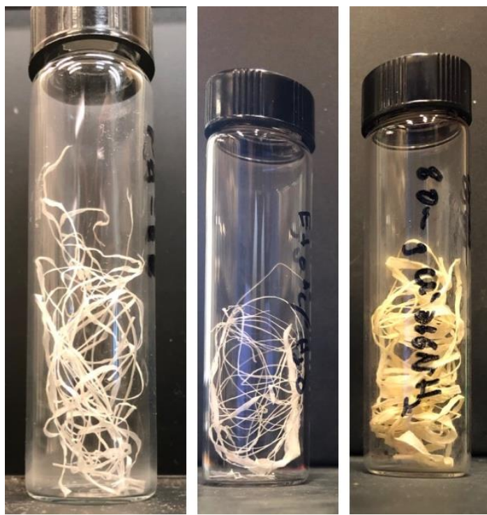
Figure 2S.15. Left: Image of PA-66. Middle: Image of PA-66@UiO-66 fiber. Right: Image of PA-66-UiO-66-NH 2 fiber.
