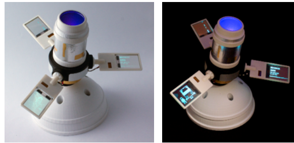
Figure 6. Overhead (illuminated and in darkness) communicating location by pan/tilt and displaying detailed satellite facts on its clear screens during each orbital flyover.
