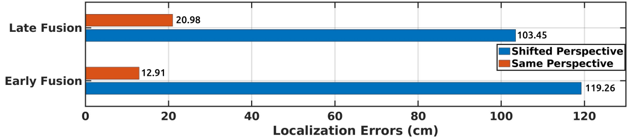
Figure 2.1: Performance degradation due to sensor perspective shift.
