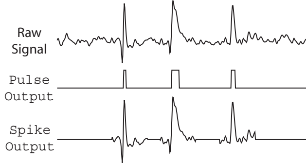
Figure 4.2: Outputs of spike detector for each mode of operation. In Pulse Output mode, a pulse is outputted each time the waveform crosses the threshold. In Spike Output mode, spike samples are outputted for subsequent spike sorting.
