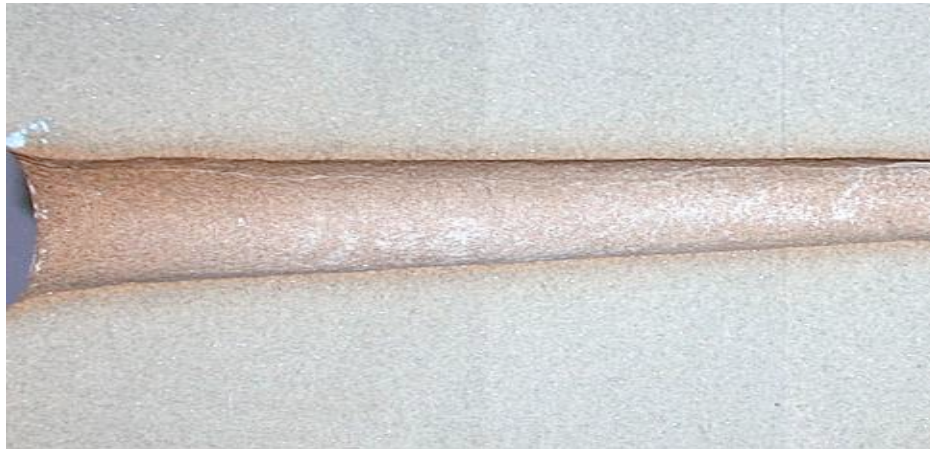
Figure 49 Perforation Tunnel in Limestone Using the Variable Focal Length Technique
