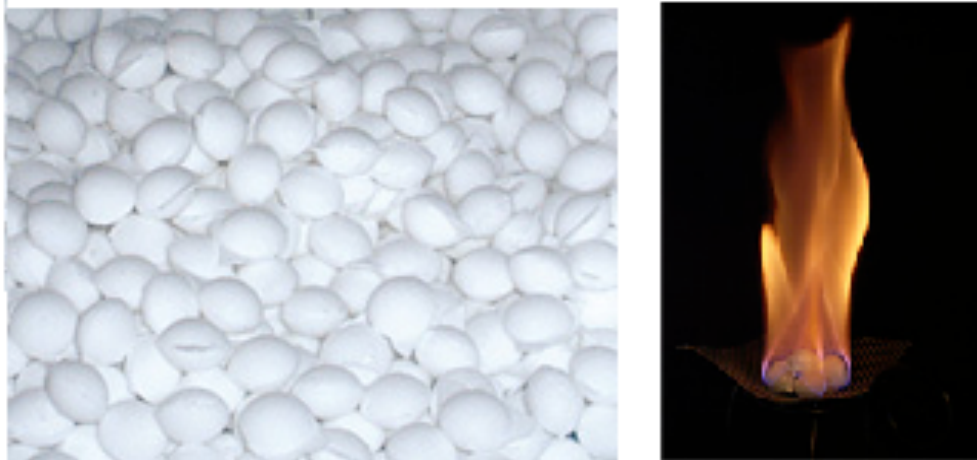
Figure 69 Photographs of NGH pellets produced by Mitsui Engineering
