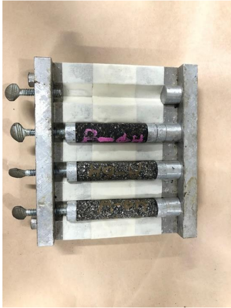
(a) Gluing FAM specimens to steel caps
