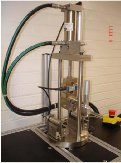
(a) I-FIT fixture
