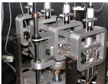
Figure 2-3 4PB testing configuration
