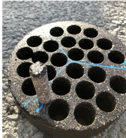
(b) A FAM mix specimen cored from the cylinder
