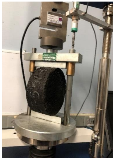
Figure 4-7 Testing machine for IDEAL-CT with a specimen
