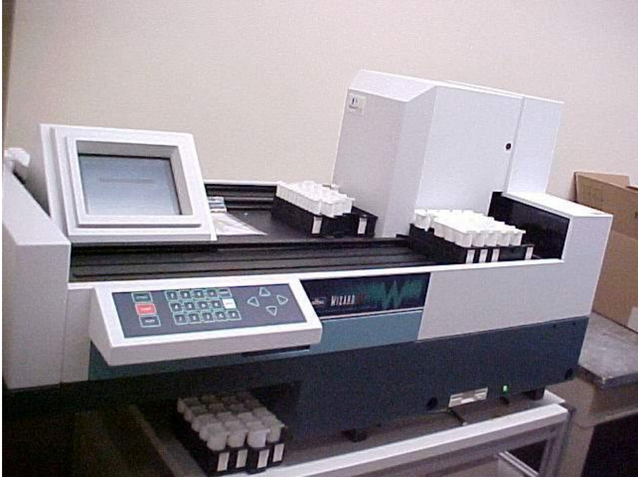
Figure 1. 3 A gamma counter that is used for measuring gamma radiation emitted by a radionuclide.
