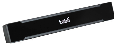
Figure 2.7: Example of Screen-Based Eye Tracker - Tobii Pro X2 eye tracker 3
