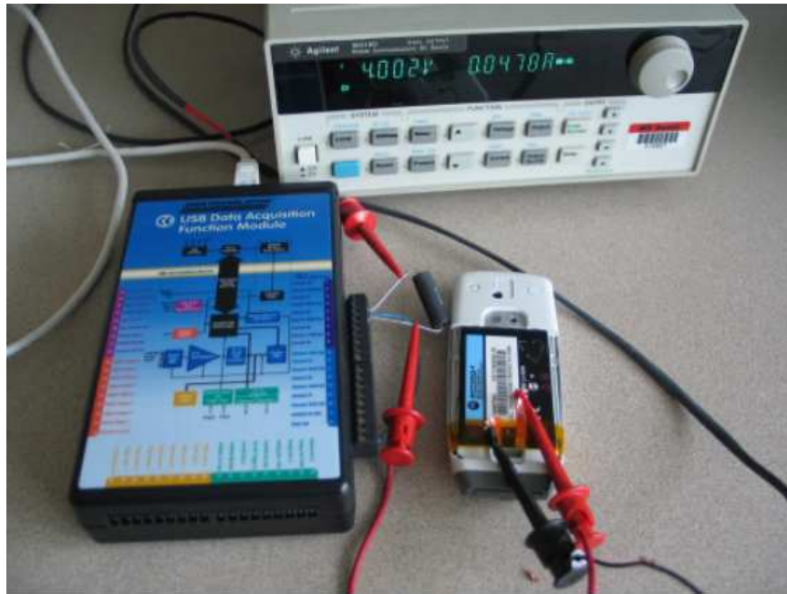
Figure 3.3: Smartphone power measurement setup
