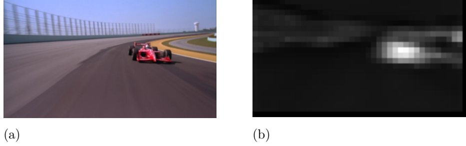
Figure 2.1: Discriminant Saliency map using dynamic texture model, (a) input frame from “Speedway” sequence, (b) saliency map. Larger pixel intensity (closer to white) represents higher saliency value.
