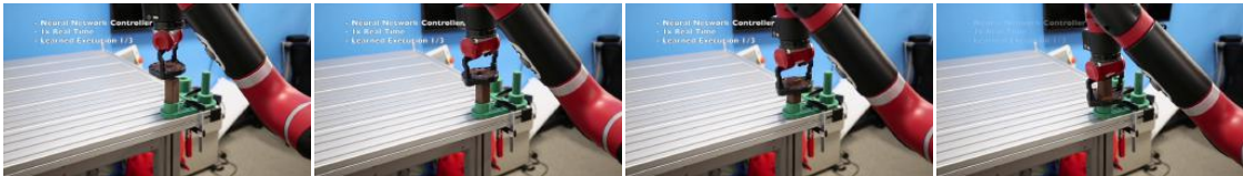
c) Task 3: Squared hole on squared shaft.
