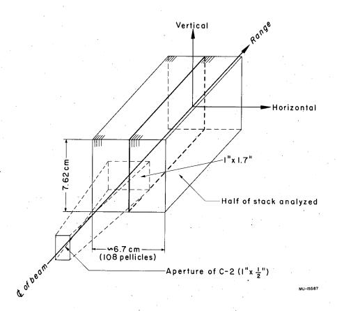
Fig. 4. Geometry of beam and emulsion stack.
