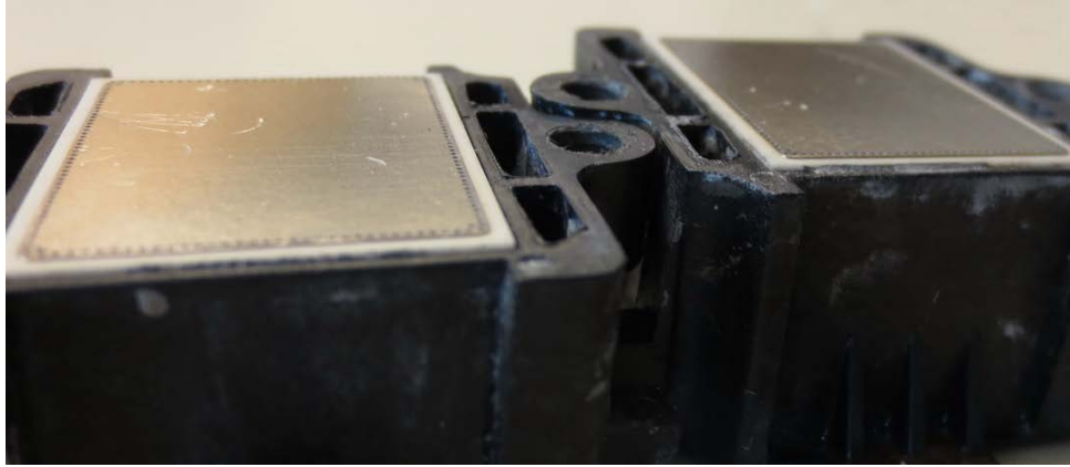
Figure 2.12: Developed Surface defects arising from continuous use
