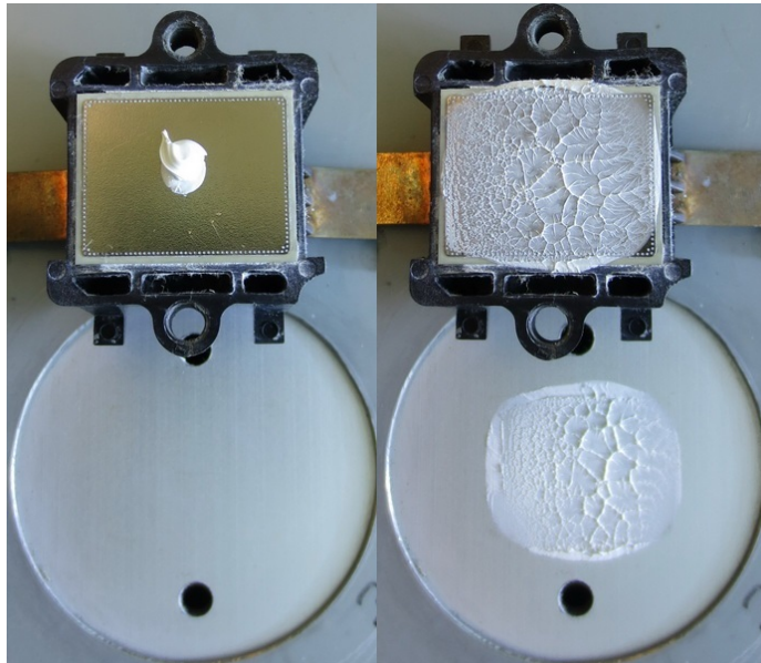
Figure 2.7: Typical spreading of thermal interface material
