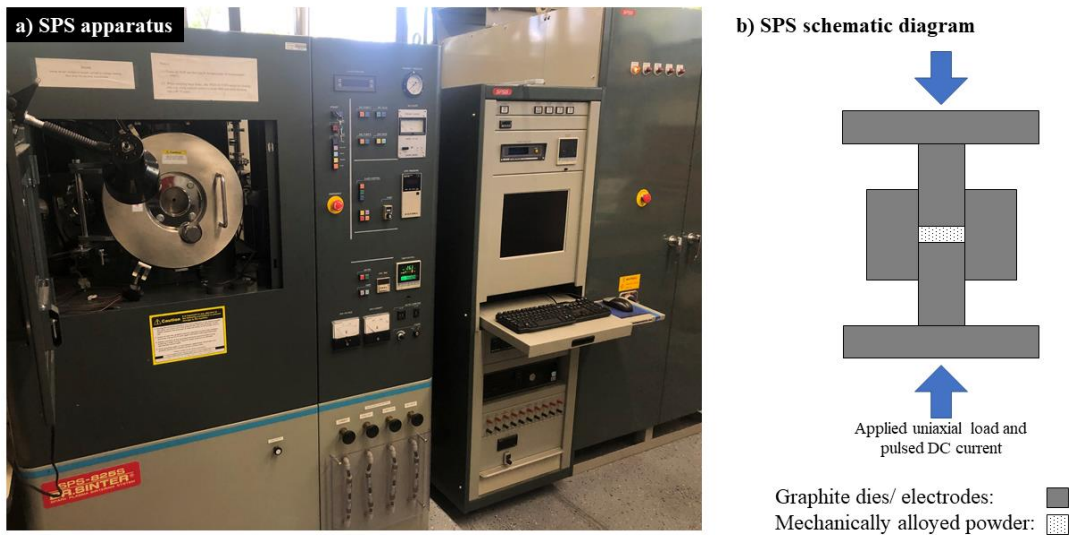
Figure 5. A spark plasma sintering (a) apparatus and (b) a schematic diagram of the components, powders, applied current, and applied uniaxial load involved in the process.
