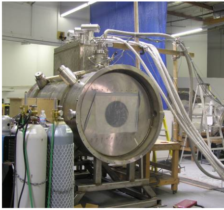
Figure 7: Spectrometer Solenoid being cooled down at Wang NMR. The first magnet will be delivered to RAL this summer.
