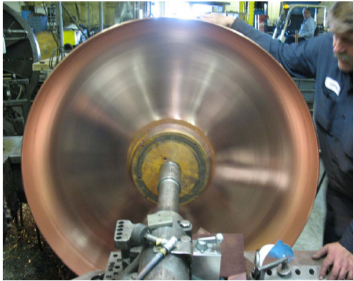
Figure 8: Cavity half-shell being prepared at Acme Metal Spinning Company.
