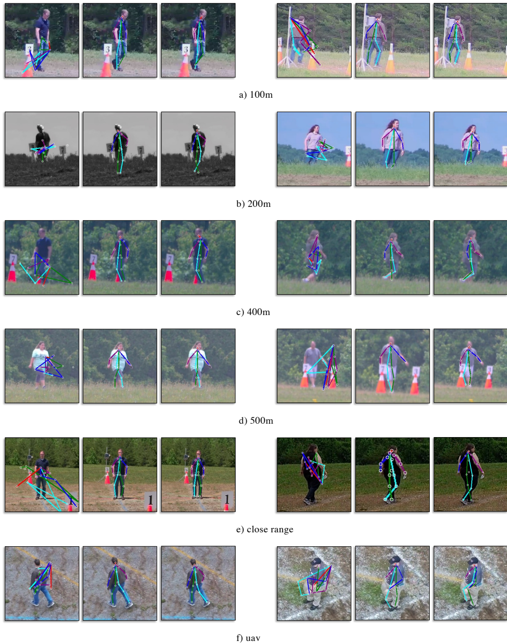
Figure 3.4: Qualitative results on SURREAL \rightarrow BRIAR. We demonstrate sample results on the BRIAR dataset at all ranges. For each range, we display three images: the leftmost shows the Source only prediction, the middle one shows the UDAPE [86] prediction, and the rightmost shows the prediction made by our framework. Although our approach does not use any source data for adaptation, it is able to match the predictions produced by UDAPE, which uses source data.
