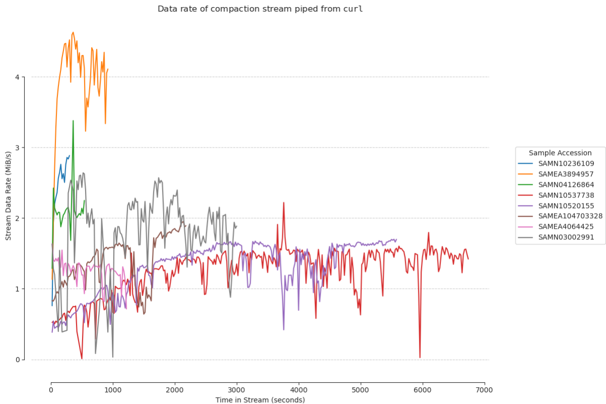
Figure 1.2: Streamed compaction data rates of various samples. Paired-end samples were streamed directly from the European Nucleotide Archive (ENA) using the curl command. The data rates were measured using the pv command as follows: curl -sL [URL] | pv -tbn 2>> [RESULTS] 1>> [OUTPUT] . [OUTPUT] is a unix pipe read by goetia cdbg build ; data rates were aggregated at 5 second intervals between both the left and right hand sample results. Higher data rates correspond to higher compaction rates and better performance. Performance here is bottlenecked by either the download bandwidth or the compaction rate, whichever is slower. SAMEA3894957 is an outlier here, with a higher download rate at the time of testing, and being a relatively small S. cerevisiae genome.
